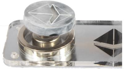
**CONCLUSIONS:** The superconductor moves freely as long as the magnetic field inside it (magnetic flux) stays the same.
