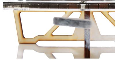
**CONCLUSIONS:** Moving around in circles is possible due to the circular symmetry of the magnetic field. In all other directions the superconductor is locked. The levitation can, thus, be easily transformed into suspension.
